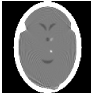
Figure A.10: Filtered backprojection reconstruction
